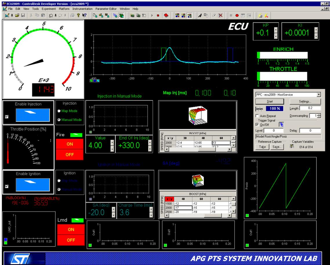
The “Kp” and “Ki” numeric inputs (on the top-right of the layout) allow to set the PI controller for motored throttle body. The “THROTTLE” slider allows to modify the throttle opening.
