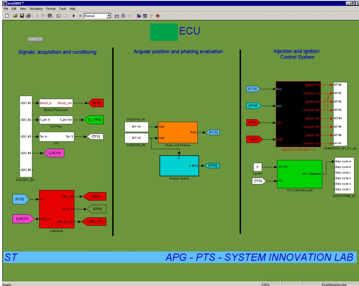
The intake manifold pressure, the in-cylinder pressure sensor signal, the lambda signal and throttle position signal were acquired using DS2001 dSPACE board, which is the board used for analog signals; on the contrary the engine speed sensor signal and Cam sensor signal were acquired by means of DS2201 dSPACE board, used for on/off signals. The project has been implemented in just one task that can be divided in several steps:
