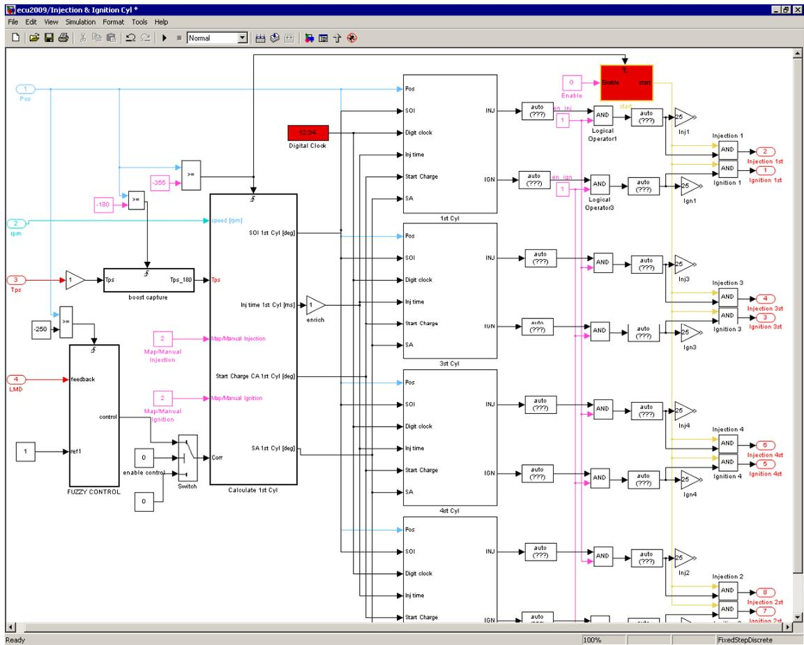
When the engine is warmed and the lambda sensor is ready to use, the ‘Lambda’ block filters the lambda signal, evaluates the error referred to the reference value (=1 typically), and gives these values to ‘ECU’ block that using a fuzzy controller modifies the injection duration in order to have a lambda = 1.
