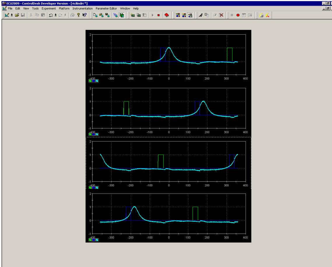
In the picture below the same  $xy$  plot related the different cylinders in the sequence 1-3-4-2 are shown. The combustion pressure sensor is installed only in 1<sup>st</sup> cylinder camera, so the other shapes are obtained from this one with a delay of 180° from the previous.
