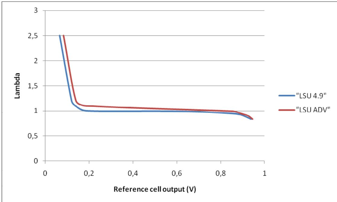
The following charts are a comparison between the Ip/Lambda characteristic present in the LSU 4.9 and LSU ADV DS and the one measured in the laboratory:
