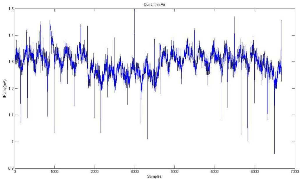
In average for LSU 4.9 the pumping current is 3,45 mA that results higher than the one certified in the datasheet. Bosch is executing some test in their Germany laboratory to check if this is due to some problem of the specific sensor sample. For LSU ADV the average current is 1.3 mA in accordance with the Datasheet value.
